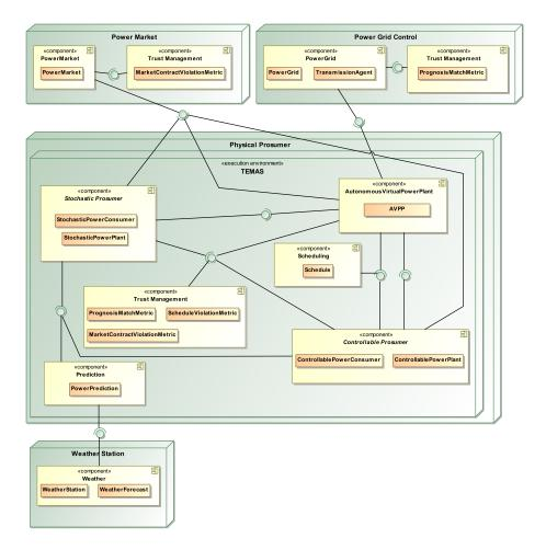
Figure 2: Components of a Trusted Energy Grid
