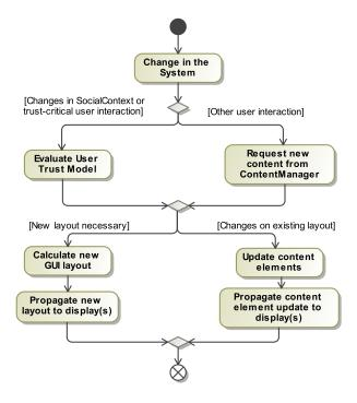
Figure 6: Based on information provided by the context, control is delegated to either the ContentManager or the UserTrustModel.
